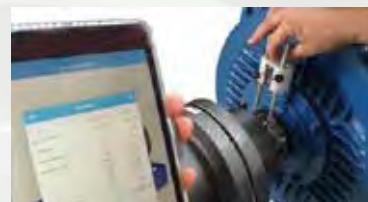
Computerized alignments by SKF laser TKSA 41 device
